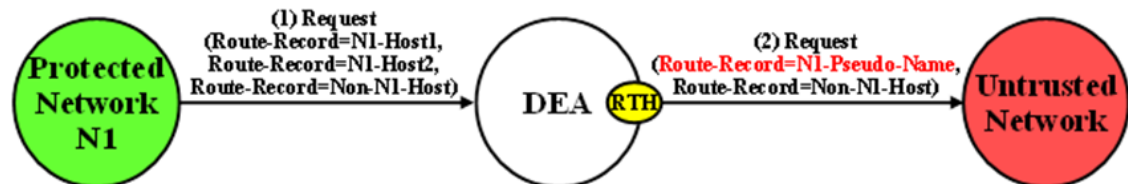
Figure 9-6 Route-Record Hiding - Request Message
